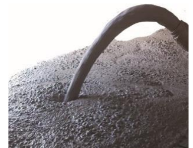
Excellent treatment ability in the absence of bleeding with w/c ratios less than 0.45
